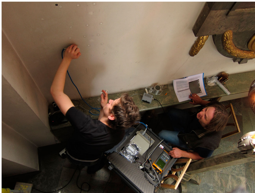
Figure 3. Ultrasonic measurement of cracks and cavities in architectural surfaces. Photo: Anna Henningsson.
